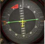
Horizontal Situation Indicator. With glideslope support and heading bug. Connected to NAV1.
