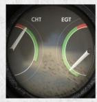
Double gauge: Cylinder Head Temperature and Exhaust Gas Temperature.
