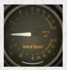
Vertical Speed indicator. Non-linear scale.
