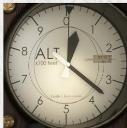
Altimeter with a QNH calibration knob.
