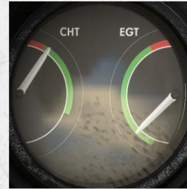
Double gauge: Cylinder Head Temperature and Exhaust Gas Temperature.
