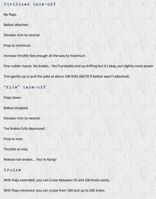
Best cruise configuration: about 100/110 knots, flaps up, prop to low and throttle to "just enough". You should get about 1600 RPMs and your fuel flow gauge should be in the blue arc. Your MFD should indicate very good fuel range and endurance estimations.
