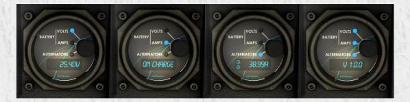
If you take too long to start the engine, or if the alternators are off, or even if the engine is not running fast enough, the battery will discharge, and systems will be shutting down one after the other. Each circuit has its own minimum required voltage.
