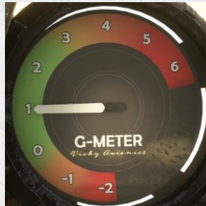
G-Meter. If you go in the dark orange, LEDs will turn on and an alarm will ring in the plane.
