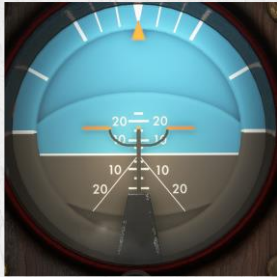
Attitude Indicator, with horizon level calibration.
