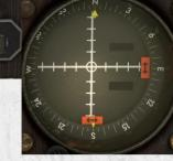
Course Deviation Indicator. With glideslope support. Connected to NAV2.
