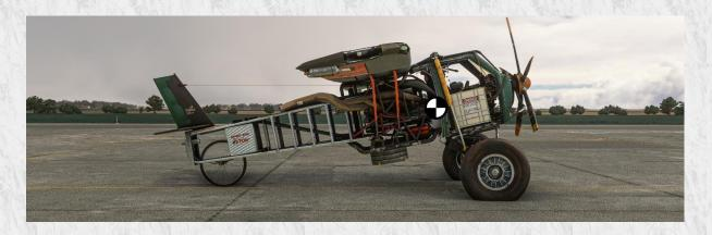
Also: The wings are relatively lightweight (fuel tank is located where the passenger seat would be in a normal aircraft). The weight is then not only centered on the roll axis, but also on the pitch axis. With all that, you end up with a plane capable of doing aerobatics quite easily.
