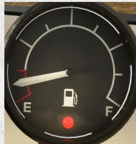
Fuel gauge with low fuel indicator light.
