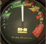
Propeller RPM indicator.
