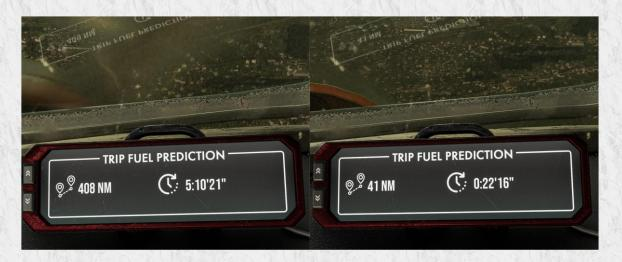
Two pictures taken at the same time, with the same fuel quantity, same everything... Only difference is one has very little throttle input and the other one is at max manifold pressure. Can you quess which is which?
