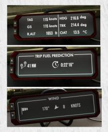
Precision navigation page. Note that the radar altimeter only works below 2000 ft AGL and with the wings roughly leveled.
