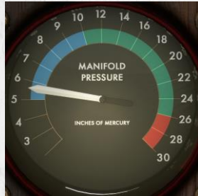
Manifold Pressure indicator (throttle).
